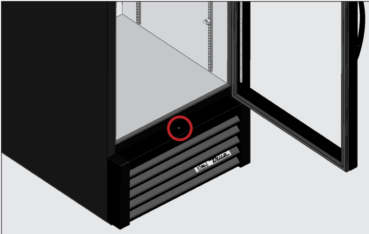
Fig. 1. Swing door lower grill screw location.
