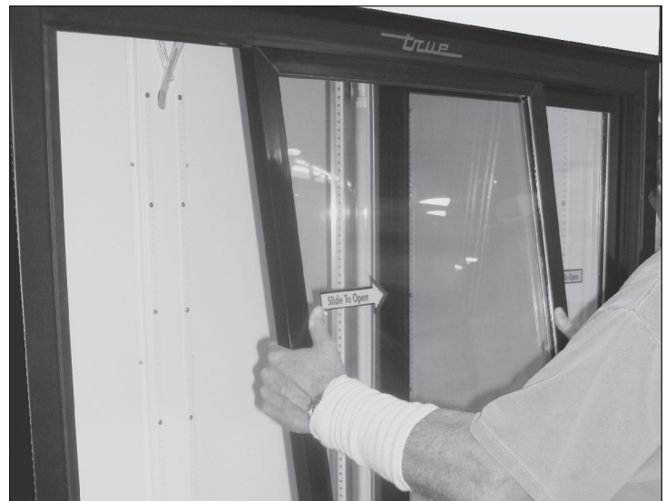
Fig. 4. Carefully remove the door.
