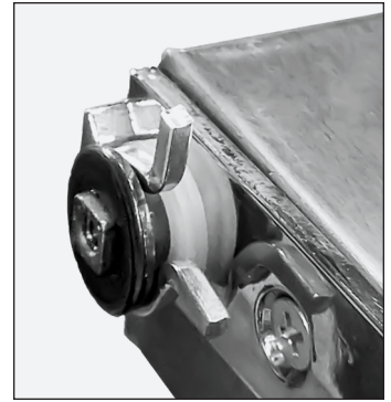
Fig. 7. Keep the washers in their original order.
