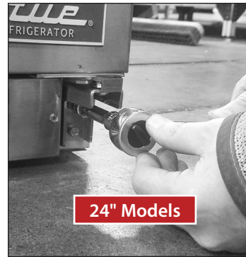
Fig. 1. The 24 and 27 models use different lower hinges.
