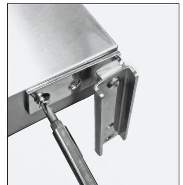
Fig. 5. Remove the cartridge hinge assembly.
