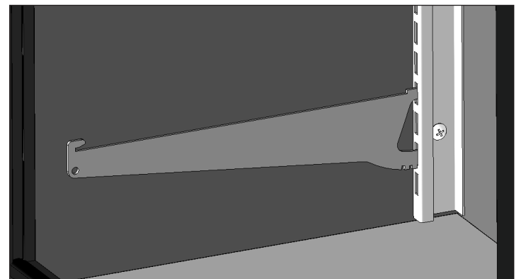
Fig. 4. Installed shelf support bracket.
