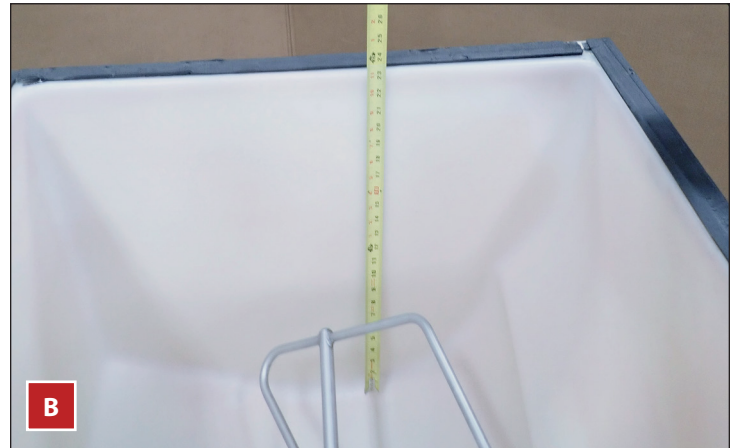
Fig. 2. Always measure the bin (A) or dispenser (B) for the ice level sensor before mounting the ice machine.
