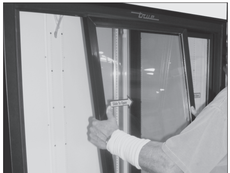
Fig. 4. Carefully remove the door.
