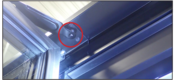
Fig. 5. Shelf shipping bracket location. One bracket shown.
