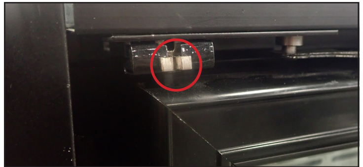
Fig. 6. Hinge retention clip installed in the top hinge. Compress the clip with pliers and pull.
