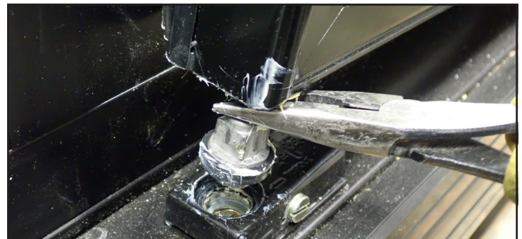
Fig. 8. An assistant lifting the torsion rod from the torque master hole while the technician lifts the door.
