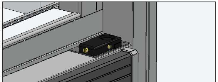
Fig. 27. Correctly installed replacement torque master assembly.
