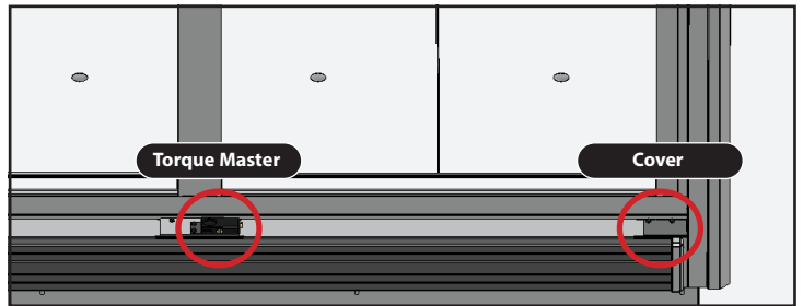
Fig. 25. Original torque master assembly and cover locations.
