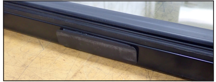
Fig. 17. Wire cover located in the hinge-side of the door in the center.
