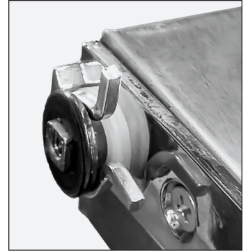
Fig. 7. Keep the washers in their original order.
