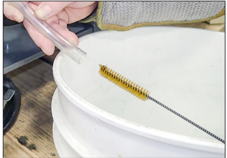
Fig. 2. Catch trapped liquid in a large container.
