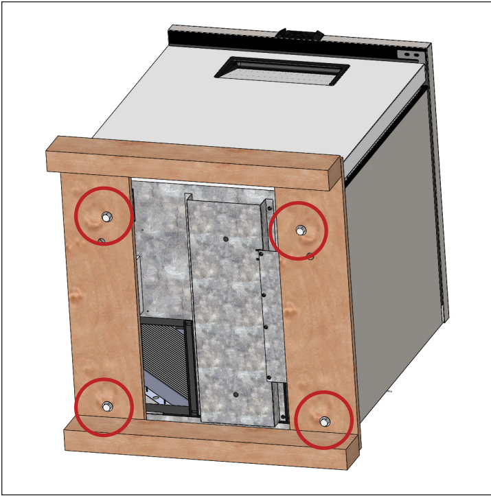
Fig. 3. Remove all shipping bolts.
