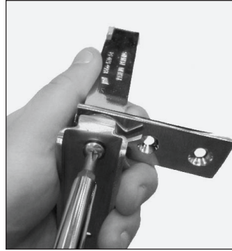
Fig. 6. Remove the hinge bracket from the cartridge spring and then rotate it.
