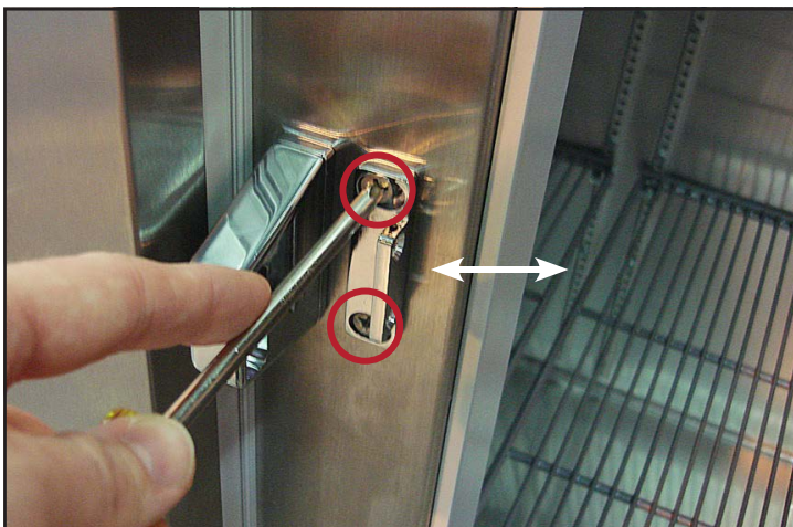
Fig. 6. Lock the base screw locations. Adjust the lock base sideways
