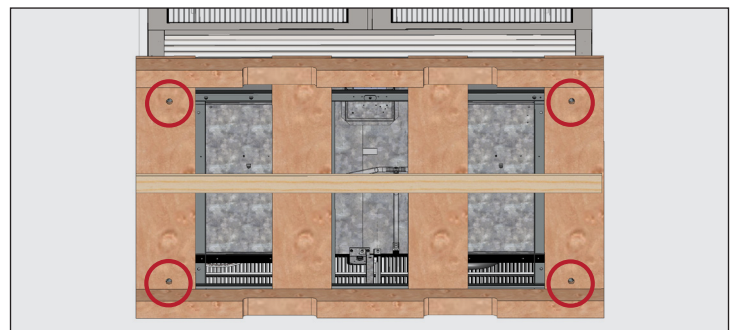
Fig. 4. Shipping bolt locations.
